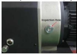
Inspection hole with G1" plug: Check the coupling and fan through this hole regularly. (The endoscope (WireCam) can be used with Smart Phone software)
